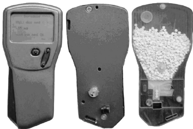
Fig. 13. Electronic dispenser for mini-tablets (Bredenberg et al., 2003).
